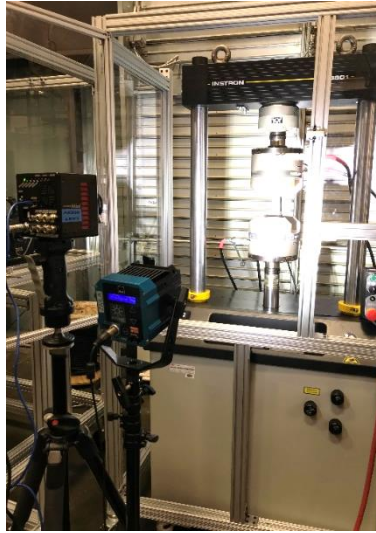
Figure 2.12 Experimental setup for testing at 50/s fastest shear strain rate
