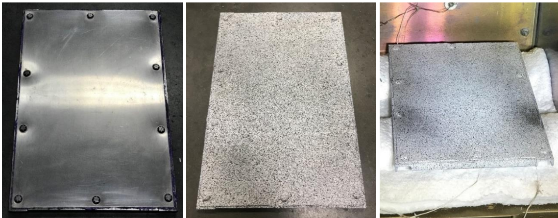
Figure 2.21 Specimen with adhesive and friction element welds
