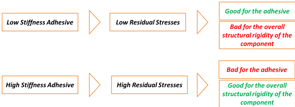
Figure 6.4 Effect of the choice of adhesive on the adhesive bond and the body structure stiffness
