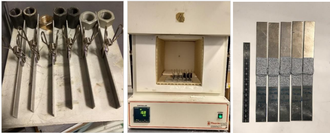
Figure 2.10 Stress free (Type I) adhesive bonded single lap shear specimen preparation
