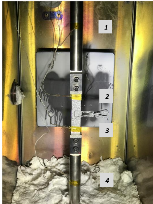
Figure 2.3 Specimen mounted on the INVAR grips and thermocouples attached at four locations
