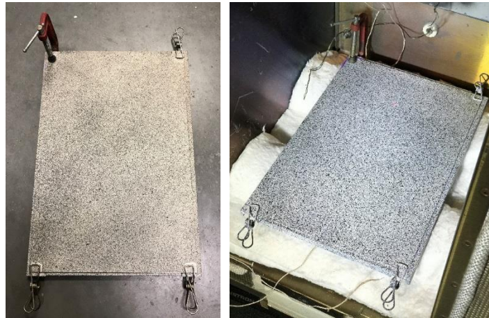
Figure 2.19 Specimen with adhesive only, hard clamped at the top left corner
