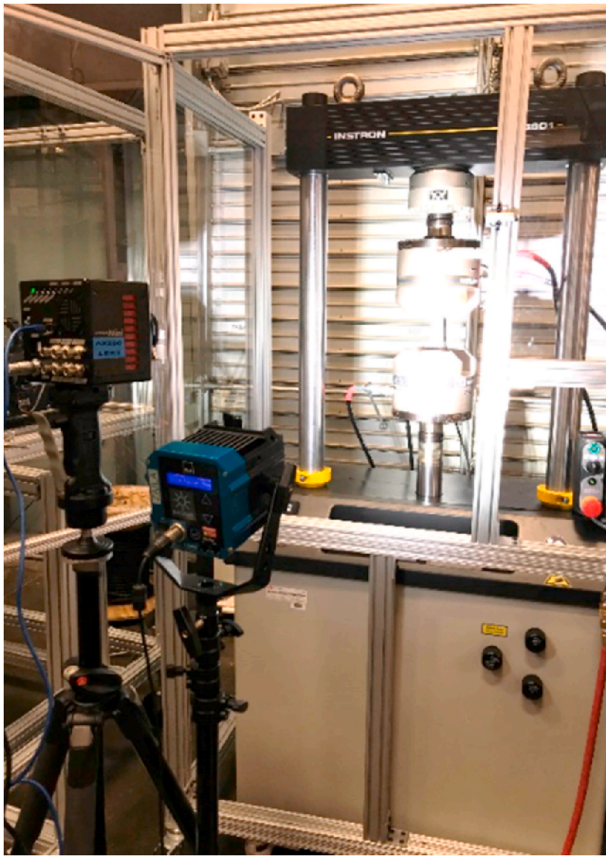
Fig. 12. Experimental setup for testing at 50/s shear strain rate.
