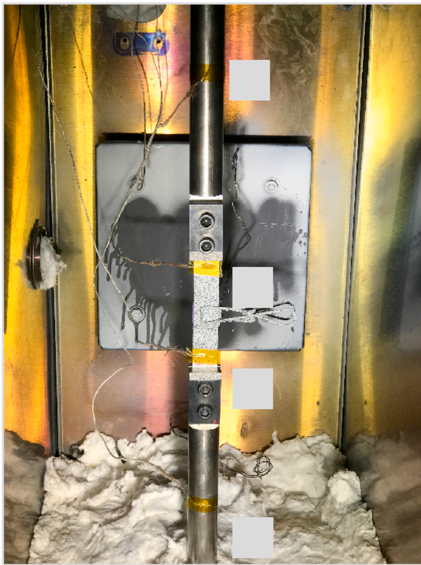
Fig. 3. Specimen mounted on the INVAR grips and thermocouples attached at four locations numbered in the figure.
