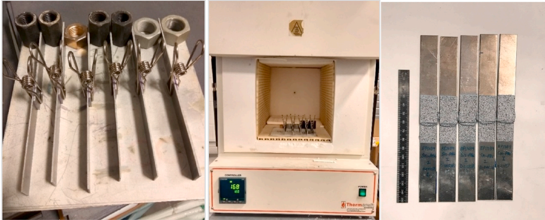
Fig. 10. Process used for producing Stress-free adhesive-bonded single lap shear specimens.
