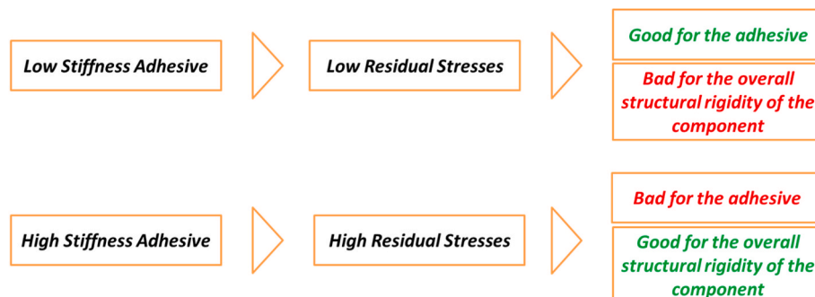
Fig. 24. Effect of the choice of adhesive on the adhesive bond and the body structure stiffness.
