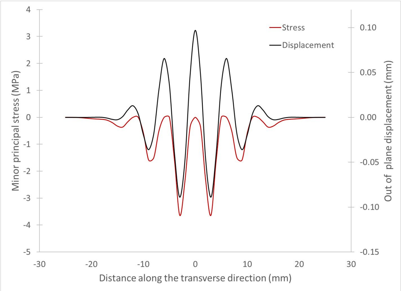
Figure 9. Minor principal stress and wrinkle profile (post buckling) along the transverse mid-plane of the membrane.
